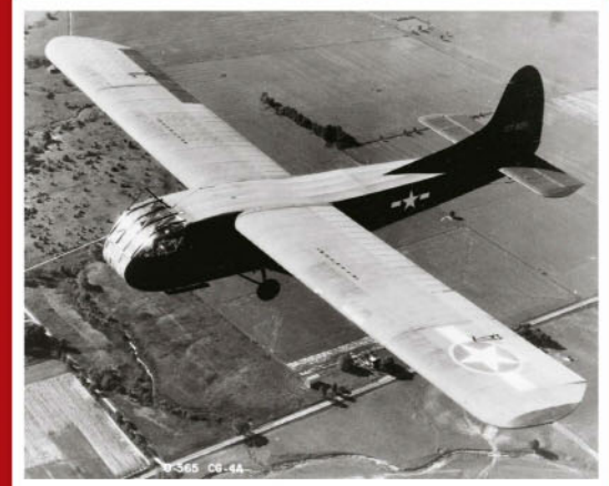
Below: The Waco CG-4 could carry up to 13 men, plus all their jump equipment
